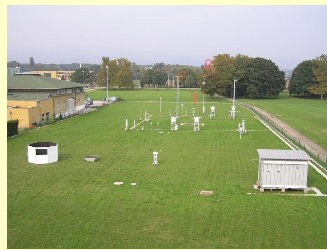
Fig. 1 The meteorological observing site at the Zagreb-Maksimir Observatory including anemometer masts of 2 m (1) and 10 m (2) of heights, respectively.
