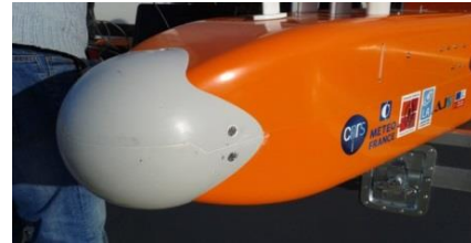
Figure 6: Picture of the five-hole probe on BOREAL
