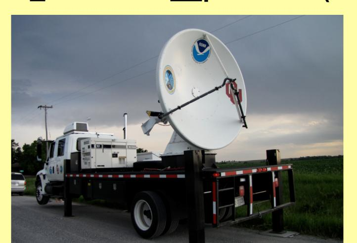
**NOAA's X-band, Dual-polarized** (NO-XP) Mobile Radar
