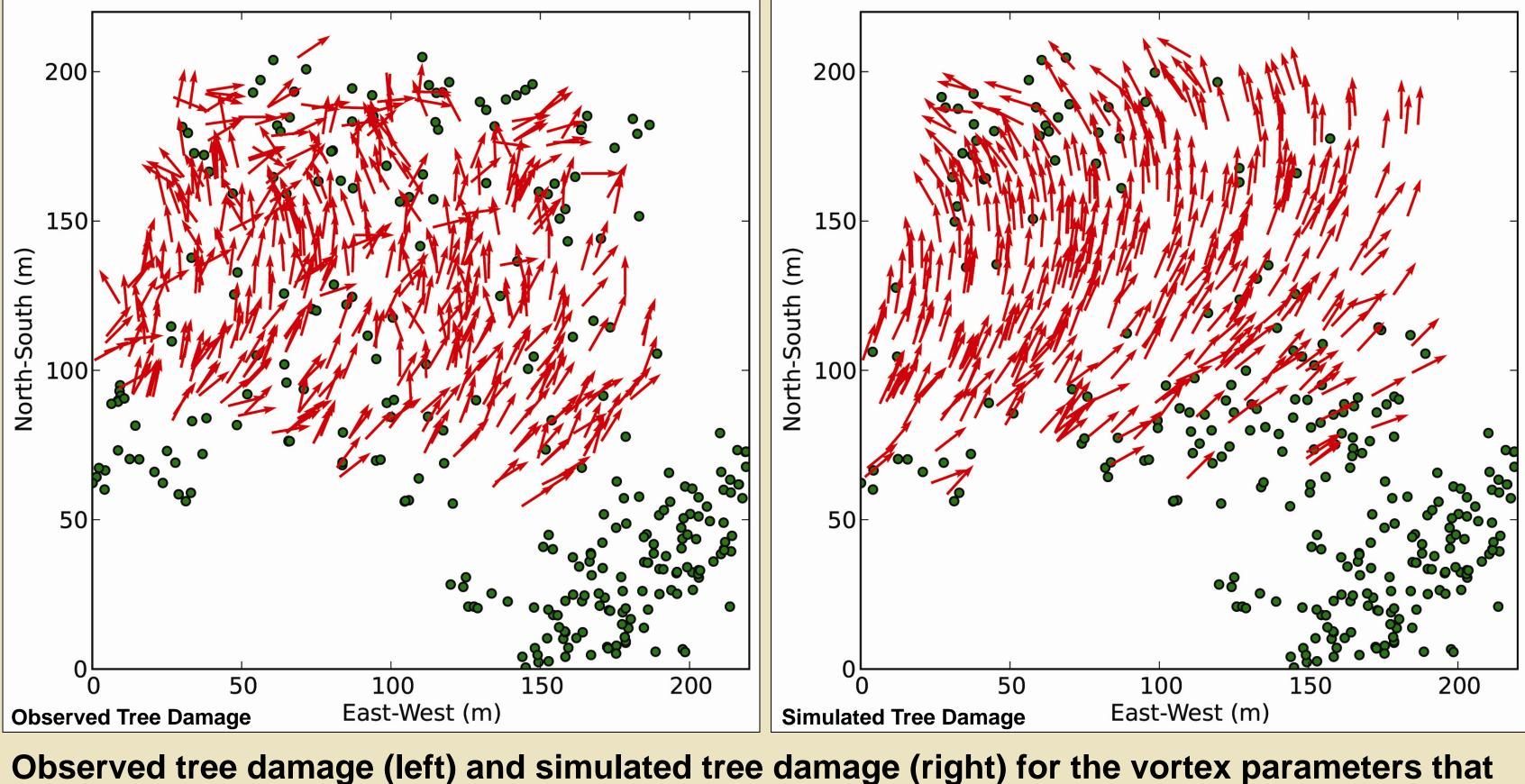
Observed tree damage (left) and simulated tree damage (right) for the vortex parameters that correspond with the maximum skill score:  $V_T = 68 \text{ m s}^{-1}$ ,  $V_R = -3 \text{ m s}^{-1}$ , and R = 40 m.
