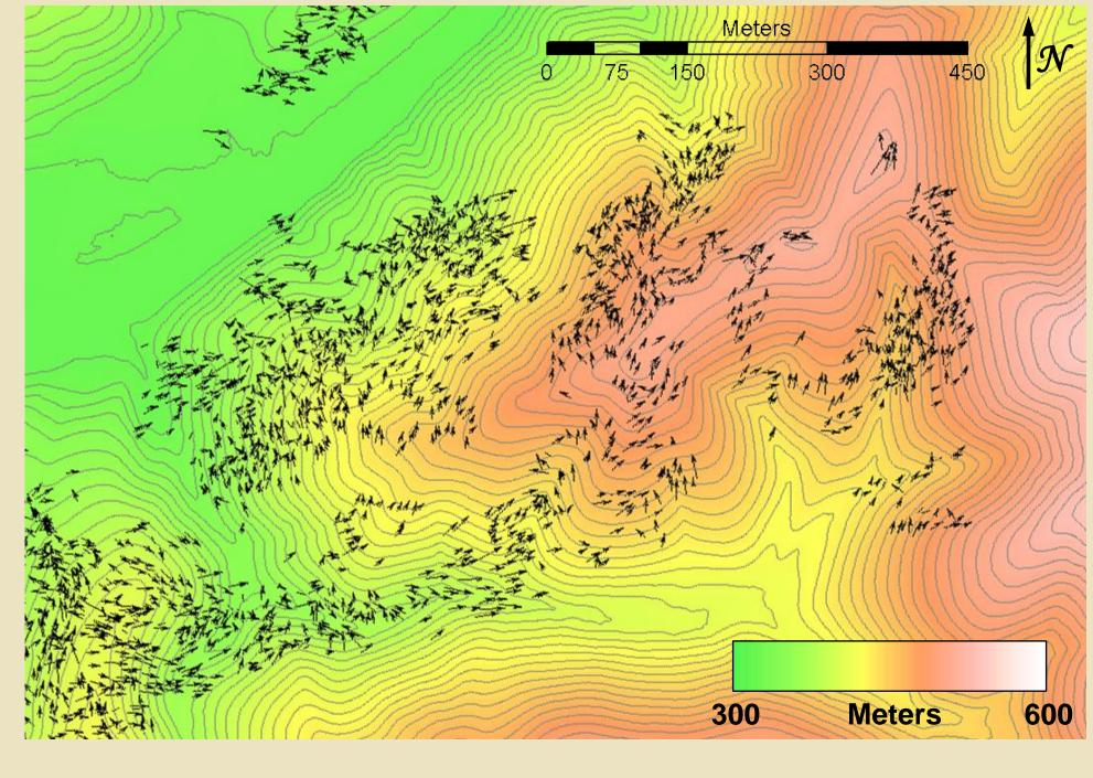
Aerial photograph (left) and treefall vectors on terrain (right). The tornado moved from the bottom left to the top right, traveling parallel to a creek, but it ascended roughly 250 m up and over a ridge rather than following the creek bed.
