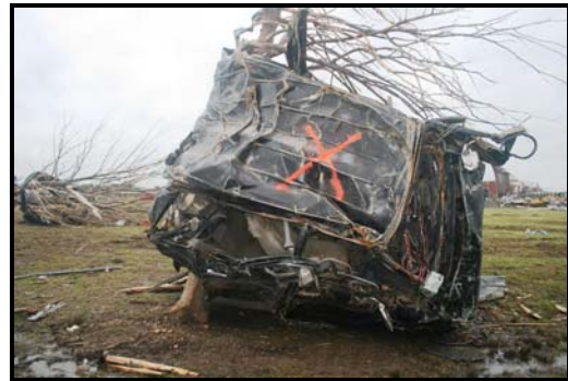
Figure 37. Four-door vehicle bent into a U-shape around a tree just south of the Walmart building.
