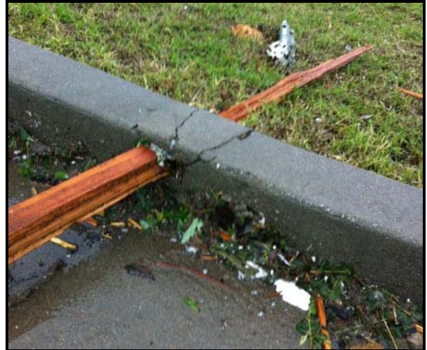
Figure 40. Wood splinter driven through a concrete curb.
