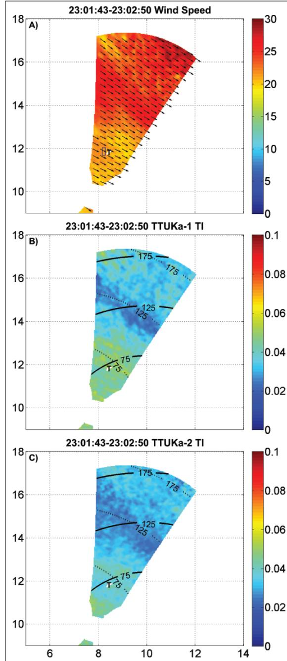
FIG. 2. (A) Dual-Doppler synthesis of radial velocity scans in Fig. 1, (B) TTUKa-1 derived turbulence intensities and (C) TTUKa-2 derived turbulence intensities. Thin rectangle, solid(dashed) contours and T denote region used for 200m tower comparison in Fig. 3, center beam height of TTUKa-1(TTUKa-2) and location of 200 m instrumented tower.
