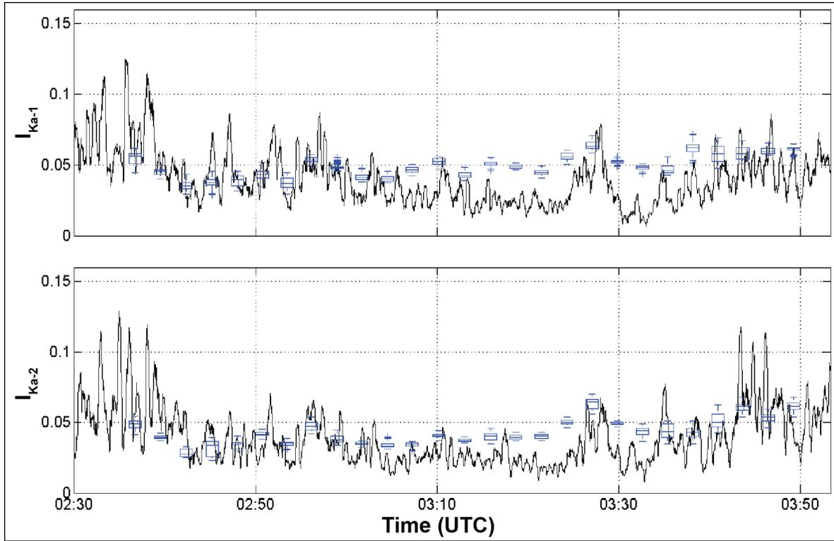
FIG. 3. (top) Time series of 74 m tower UVW turbulence intensity of the TTUKa-1 radial component of the wind with box and whisker plots of TTUKa-1 derived turbulence intensities within a 150 x 400 m rectangle upstream of the tower (Fig. 2a). (bottom) As in the top panel but for the TTUKa-2 radial component of the wind.
