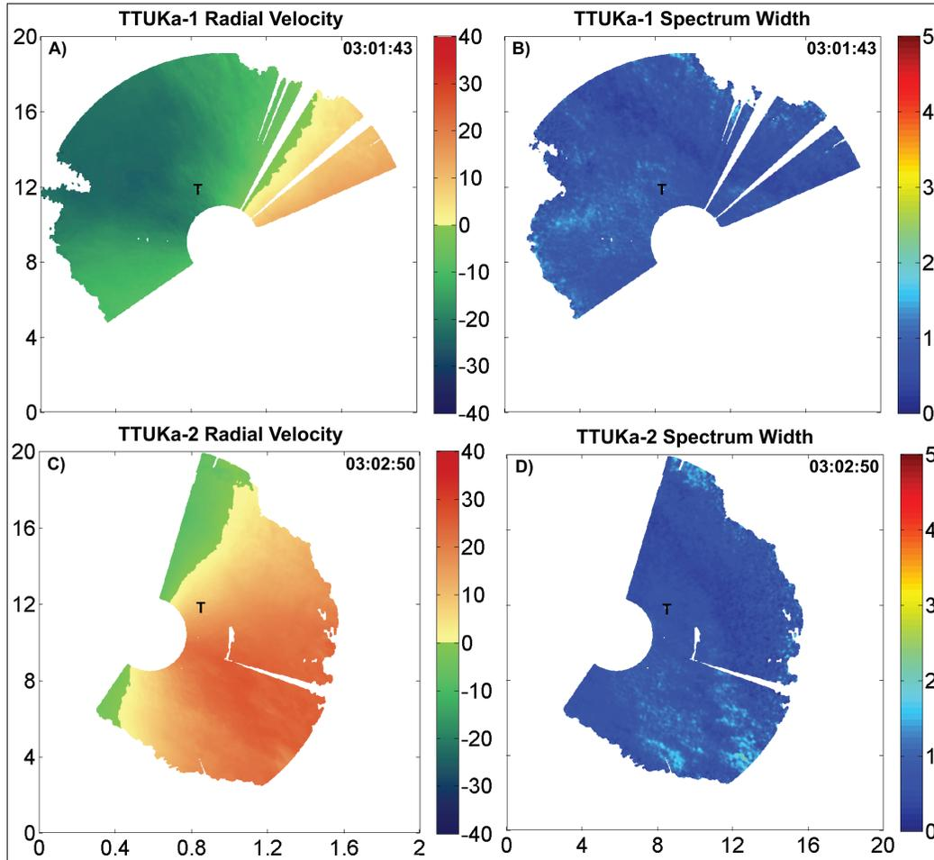
FIG. 1. Objectively analyzed TTUKa radial velocity ( $\text{m s}^{-1}$ ) (A, C) and spectrum width ( $\text{m s}^{-1}$ ) (B, D)  $1.0^\circ$  elevation angle PPIs from 15 June 2012. Bold “T” represents location of the 200 m instrumented tower.
