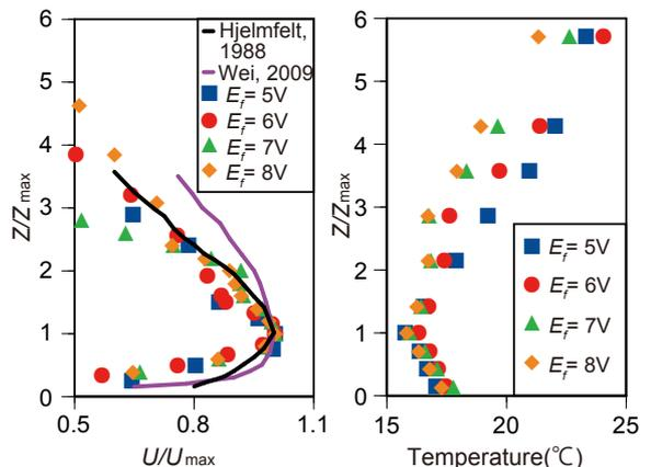
Fig. 3 Velocity and temperature profiles of simulated outflows
