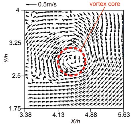
Fig. 7 Velocity field of a tornado-like vortex at  $Z/h=0.25$  ( $E_p=5V$ ,  $E_f=8V$ )
