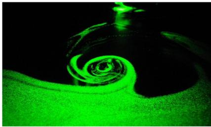
Fig. 6 Plan view of tornado-like vortex ( $E_p=0V$ ,  $E_f=6V$ )
