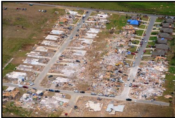
Figure 28. Aerial view of the Parkwood Meadows subdivision in Vilonia where dozens of homes were swept clean from their concrete slab foundations. This appeared to be EF5 damage. However, closer inspection from our ground survey found poor attachment of the houses to their foundations.
