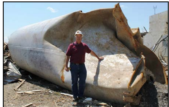
Figure 24. A large steel tank that traveled 1192 m and was found behind the strip shopping center.
