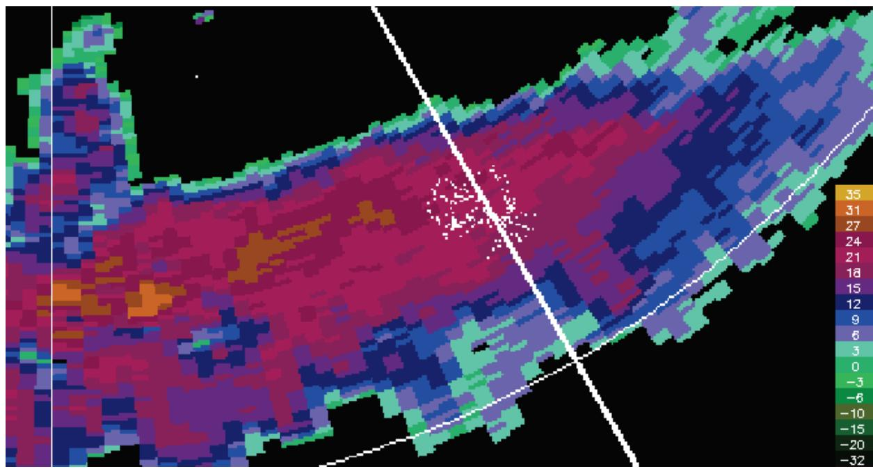
Figure 8. Low-level reflectivity (colour legend in dBZ at right) from the King City radar in Ontario at 23:00 UTC on November 20, 2014, with SOLMA sources superimposed (white dots). As shown in Fig. 7, CLDN detected a negative cloud-to-ground flash followed by a negative in-cloud flash near the same time and location as the SOLMA-detected flash.
