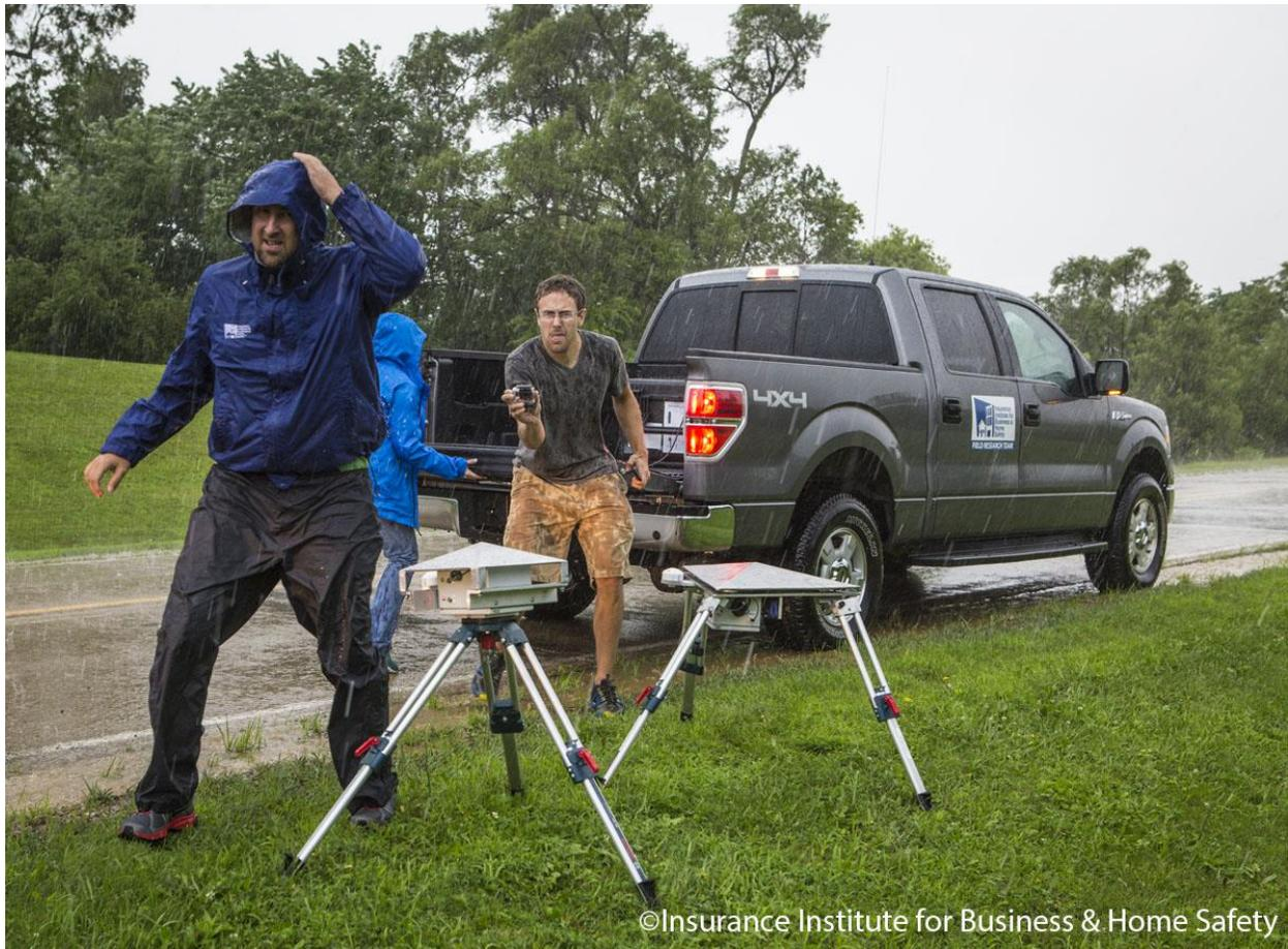
Figure 3. Photograph of the two prototype hail impact disdrometers (A-type left, B-type right), deployed during the 2014 field phase.
