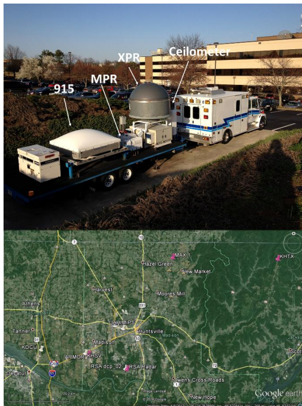
Figure 1: Picture of MIPS (top) with labeled 915-MHz Doppler wind profiler (915), multi-channel profiling radiometer (MPR), X-band Doppler profiling radar (XPR), and a ceilometer, along with a map of the northern Alabama observational array (bottom).
