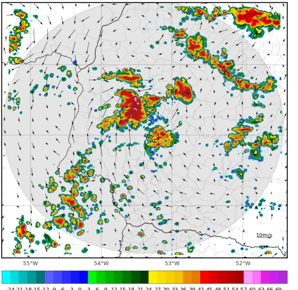
The second experiment used the M2 forecast at 17UTC as background for radar data assimilation. The side figure shows the reflectivity at 18UTC. While the model without assimilation was not able to generate the convection as observed with radar data, the high-resolution simulation with assimilation yields a development of the convection cells compared to the observations, although in some areas the simulated reflectivity were overestimated.
