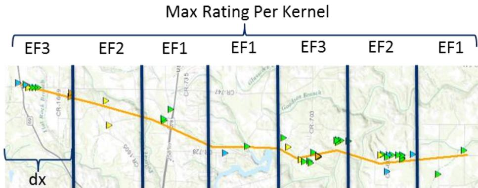
**Figure 8. Illustration of Path Discretization and Maximum DI Determination**
