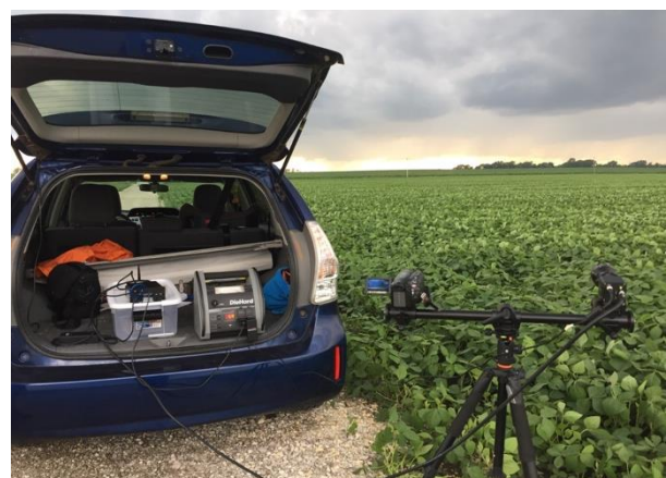
Fig. 2: The Canon HV30 HD camcorder (left on tripod) and the Goodrich GA 1280J SWIR camera (right) recording video in the 7 July 2016 Boswell, Indiana storm.
