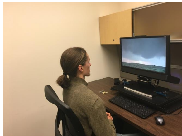
Fig. 3: A trained spotter participant observing VIS video footage of a developing tornado while using the Tobii TX300 eye tracking system. The spotter's eyes are tracked by a low-power, infrared sensing array mounted below the screen.
