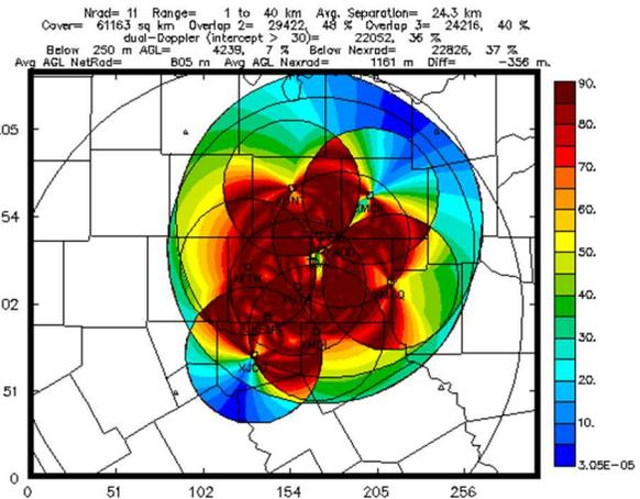
Figure 4. Maximum dual-Doppler crossing angles (color, degrees, scale at right) for combined CASA X-band (40 km range rings), TDWR and NEXRAD radar network.
