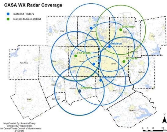
Figure 1 Map of the DFW Urban Testbed showing current status of CASA X-band Radar Network. Blue circles indicate 40-km range rings for radars deployed as of November, 2016. Green circles are for planned radar sites. Background map shows county boundaries of the North Central Texas Council of Governments.
