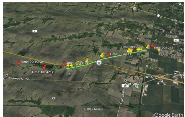
Figure 8: Map of the tornado track determined from the National Weather Service damage survey (green line), NWS damage indicators (yellow pins), and tornado location determined from the high-resolution radar data (red pins). The time (in UTC) of the radar scan is listed next to the corresponding red pin.
