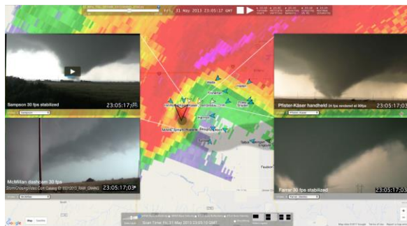
Fig. 2: Example of the web-based TED tool. Temporally and geo-synchronized video from up to 4 storm chasers can be displayed at the same time. The background image is the KTLX WSR-88D radar imagery valid at the time the videos are rolling, and storm chaser locations (blue triangles) are superimposed upon the radar image, with a Google Earth map of the area as the base layer. The user can choose which video to show in the screen by selecting the GPS icon on the background image, or selecting the user from a drop-down menu.
