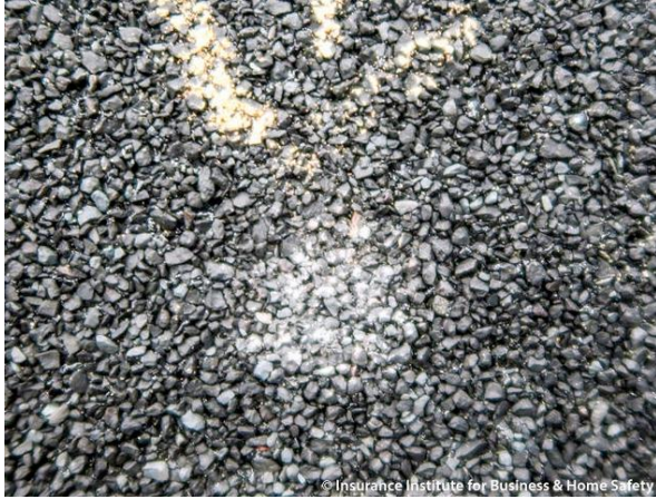
Figure 1: The steel ball utilized in UL 2218 tests crushes granules on shingles.
