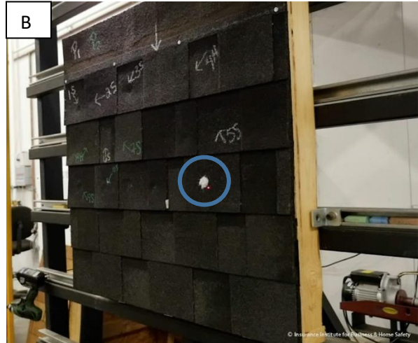
Figure 8: Soft impact mode ice spheres will break into many fragments upon impact with the test sample and will leave a slushy residue on the test panel.
