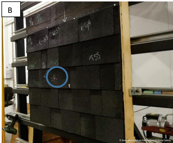
Figure 7: Hard shatter impact mode ice spheres will break into many fragments upon impact with the test sample and will not leave a slushy residue on the test panel.
