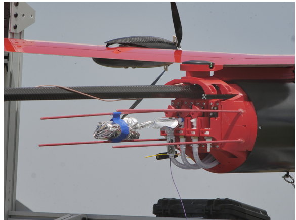
(b) ALD in the storage position behind the fuselage of the Mistral before flight. Photo credit: Cole Kenny, IRISS.
