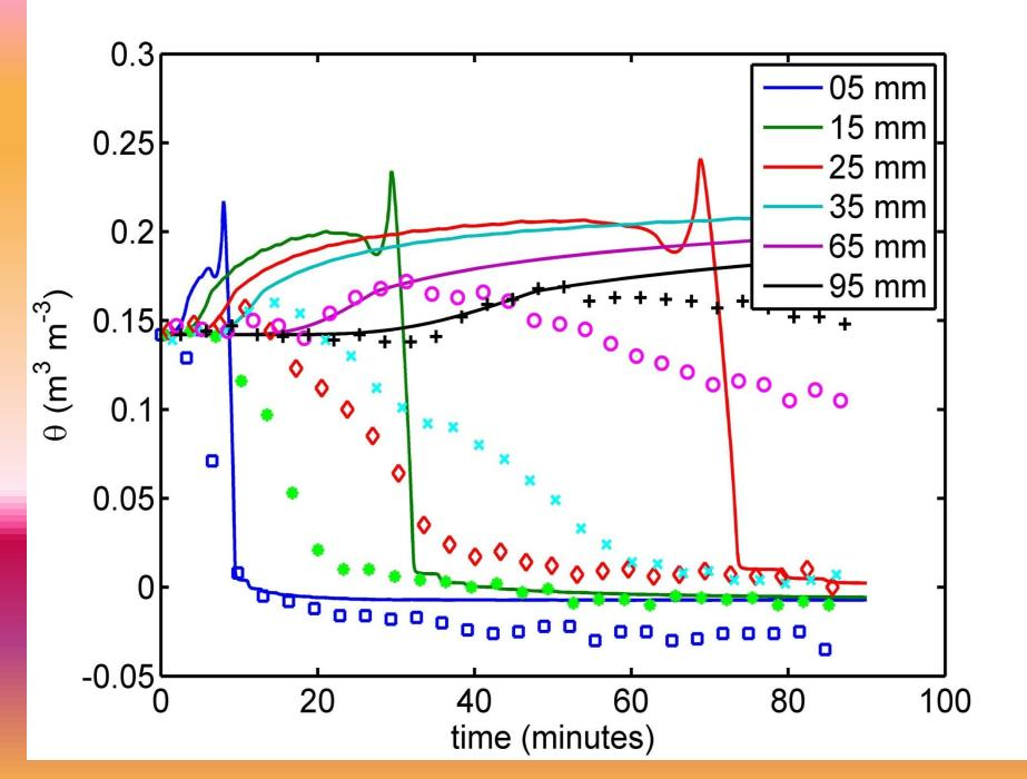
Comparisons suggest that present model provides a reasonable qualitative picture of soil moisture evaporation and heat flow during fires. But for quantitative purposes the new model may not be as accurate as the original *Campbell et al.'s (1995)* model !!
