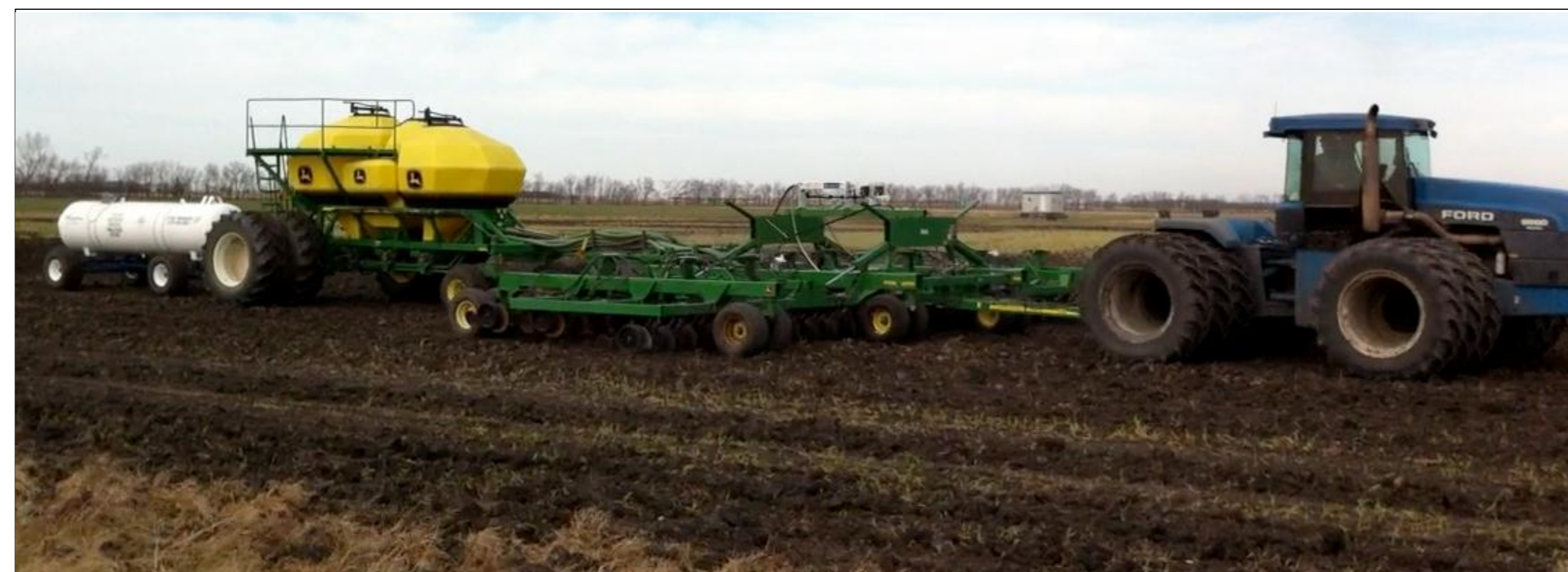
Fig. 2: Application of anhydrous ammonia in the field. Anhydrous ammonia was injected 5 cm below surface at 50 cm row spacing.
