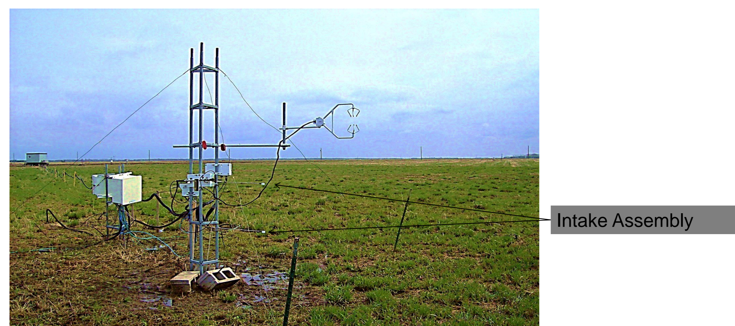
Fig.3: Instrumentation tower at the center of the plot showing gas intake assembly.
