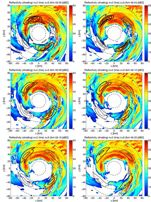
Figure 2: Horizontal cross sections at  $z = 3.2$  km of reflectivity from 09:00 to 09:20 UTC of Aug/20 at 4-minute intervals, with the positive and negative parts of its  $n = 2$  component overlaid as thick and thin black lines (only  $\pm 10, 15, 20, 25$  dBZ are shown). Dashed lines are concentric circles at every 20 km radius.
