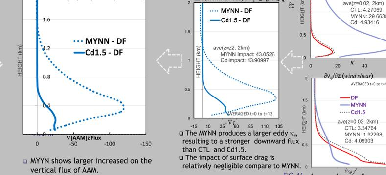
□ The MYNN produces a larger eddy  $\kappa_m$  resulting to a stronger downward flux than CTL and Cd1.5.
