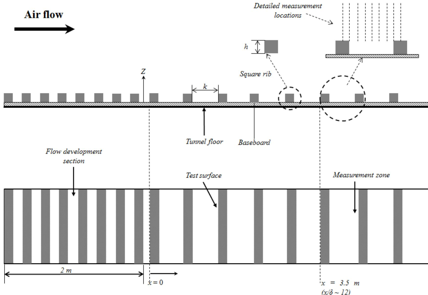
Schematic of the test rack for surfaces with idealized roughness elements used in the wind tunnel experiments.
