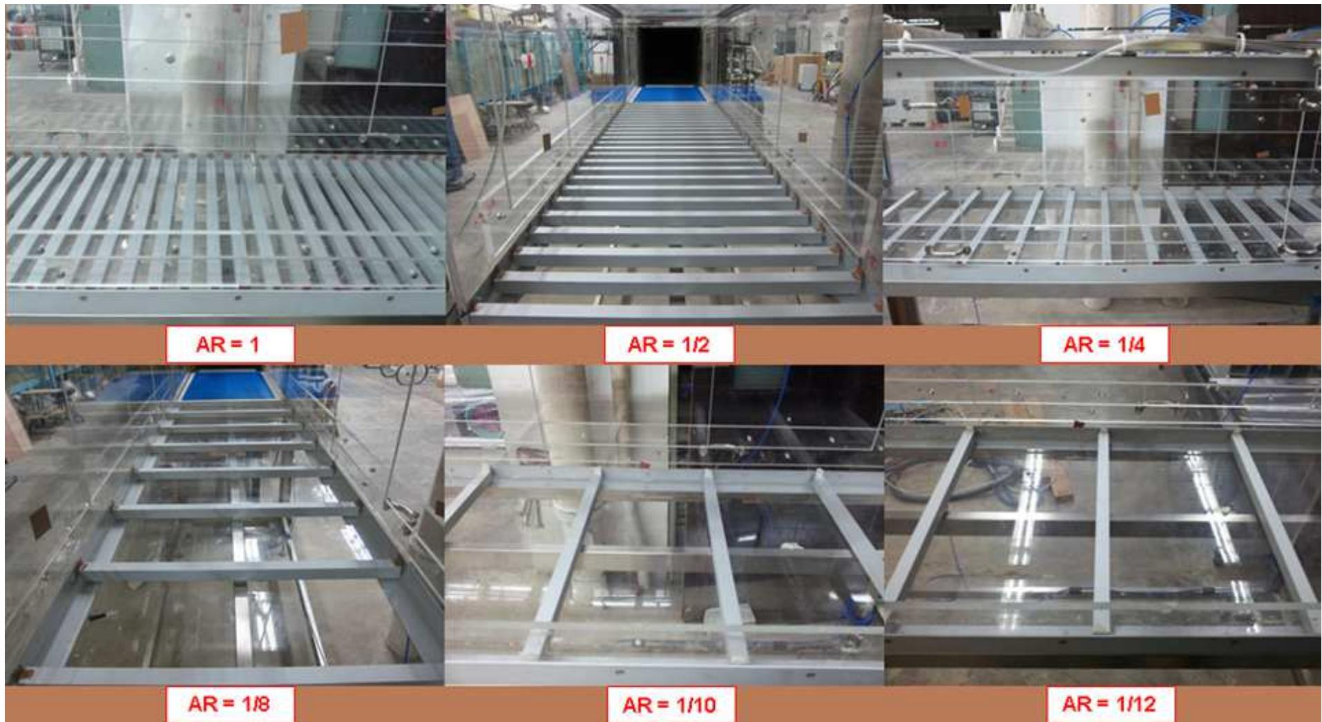
Reduced-scale models of idealized urban roughness used in the wind tunnel experiments.
