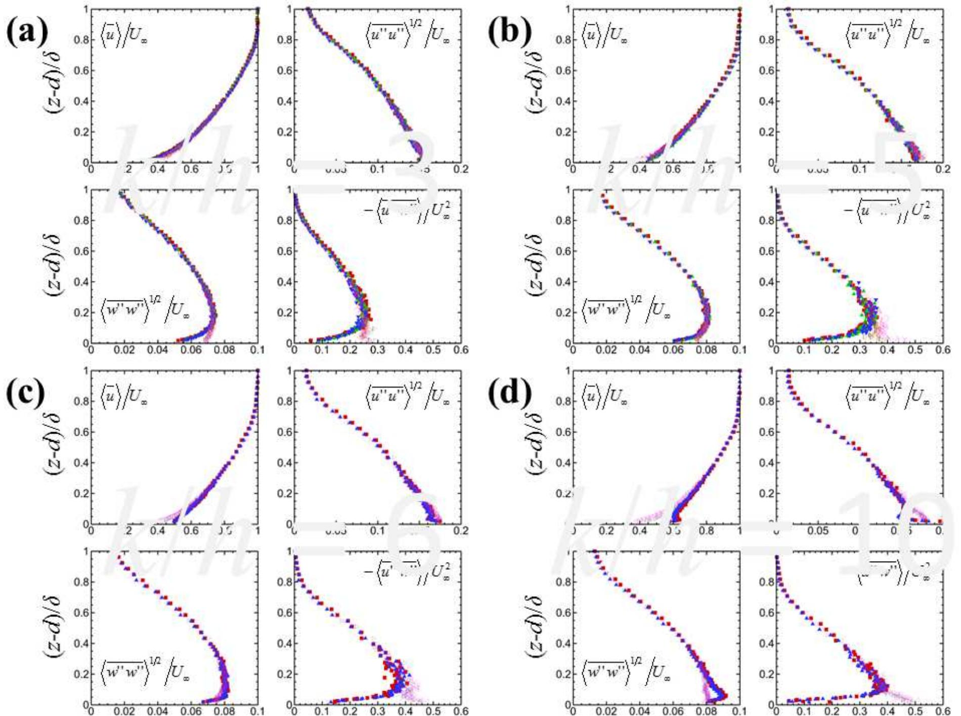
Profiles of dimensionless flow properties in the streamwise direction for different  $k/h$ . Filled & empty symbols represent, respectively, the measured profiles at the centerline of ribs and cavities.
