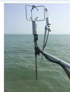
Figure 2. CO<sub>2</sub>/H<sub>2</sub>O gas analyzer and sonic anemometer
