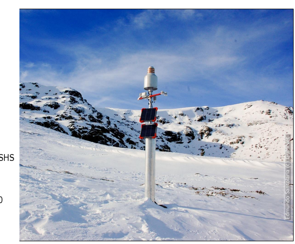
Fig 10. EG006-Hoyas automatic weather station is located in the cirque valley of Peñalara at 2.019 m a.s.l. Abounding in tall grass and wetlands the design of the station aims to minimize the impact on the environment without the perimeter security fence. A single mast houses all atmospheric instrumentation. Since it is located in an area of high snow accumulation during the winter season, the mast is configured to be over the snow cover and highly visible for ski activities.
