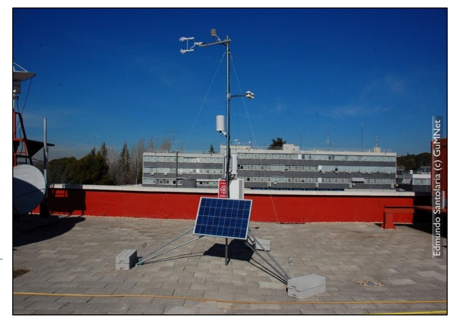
Fig 8. (left scheme, right picture) The EG901- Portátil is a portable automatic weather station design to monitor CO 2 , H 2 O and other turbulent fluxes as well.
