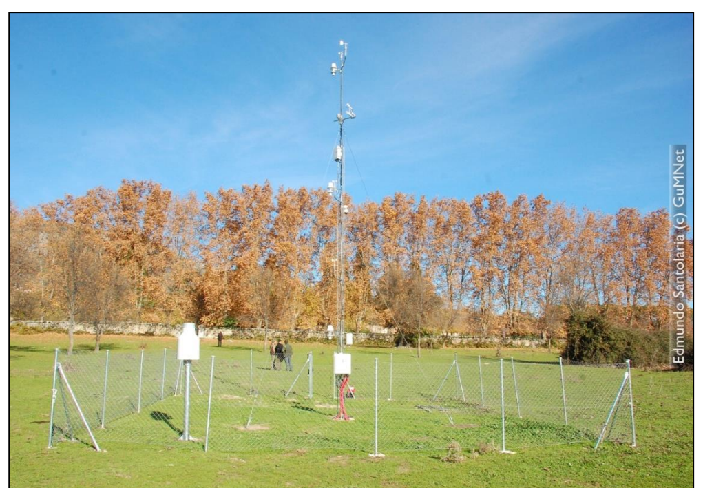
Fig 7. (left scheme, right picture) EG010- La Herreria automatic weather station is located in the municipality of El Escorial at 920 m a.s.l. Atmospheric instrumentation has been installed in order to study the boundary-layer evolution and CO 2 , H 2 O and other turbulent fluxes.
