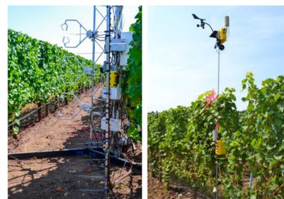
Figure 7: The TC rake & 2 LEMS deployed in the vineyard with anemometers above & below  $h$  (2014)
