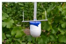
Figure 4: Rotating rod impaction trap
