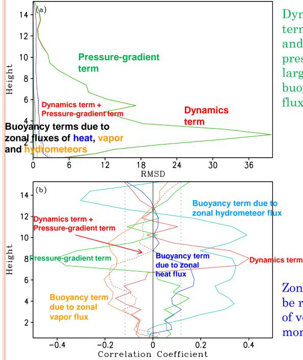
Dynamics and pressure-gradient terms are largely cancelled out, and sum of dynamics and pressure-gradient terms are also largely cancelled out by buoyancy term due to zonal heat flux
