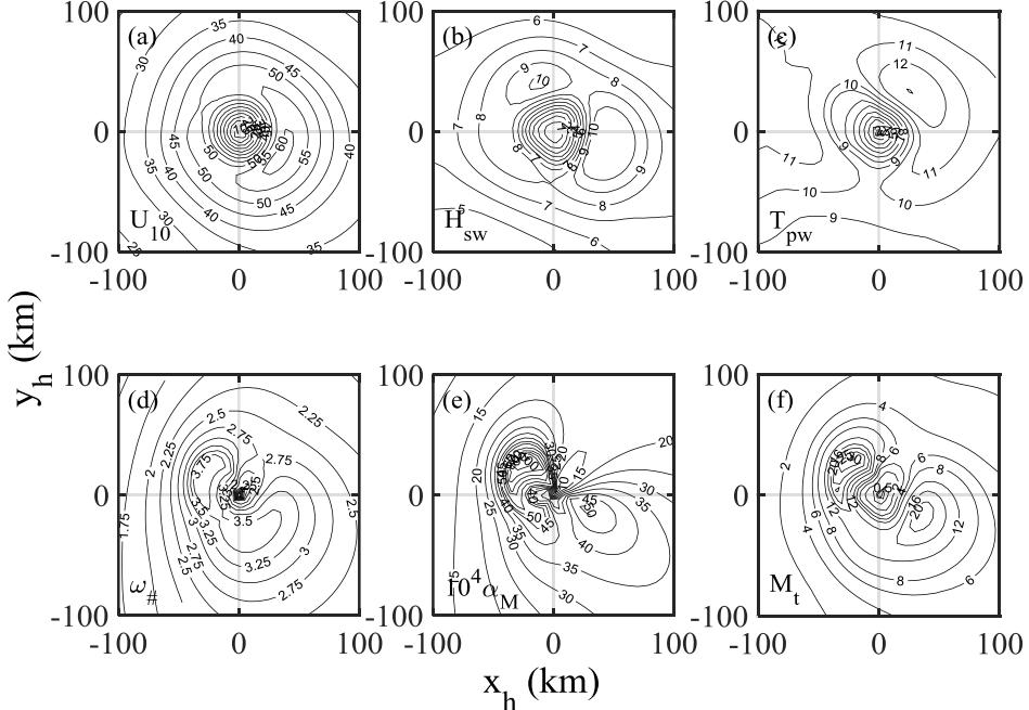
Fig. 3. An example illustrating the derivation of wave and air-sea interaction parameters using the hurricane wind field as an input, shown here are (a) input  $U_{10}$ , and outputs of (b)  $H_{sw}$ , (c)  $T_{pw}$ , (d)  $\omega_w$ , (e)  $E_t$ , (f)  $M_t$ ; subscript  $w$  emphasizes that the wave parameters derived from the fetch- and duration-growth functions are the wind sea components.
