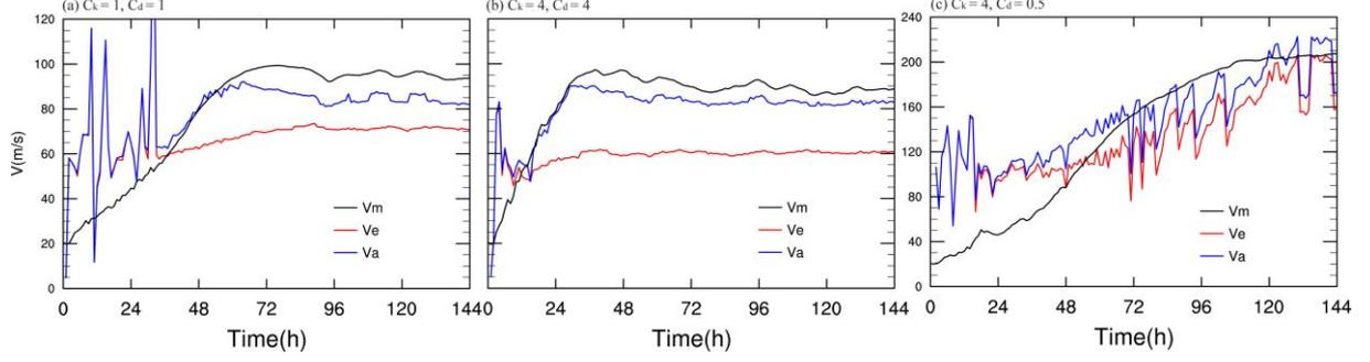
Fig. 3. Time series of  $V_m$  ( $\text{m s}^{-1}$ ) from the control simulation (black line), the velocity calculated from (1) ( $V_e$ , red line) and  $V_a$  from (2) which includes  $V_e$  and the non-gradient-wind-balance term (blue line) for a)  $C_k = C_d = 1 \times 10^{-3}$ , b)  $C_k = C_d = 4 \times 10^{-3}$  and c)  $C_k = 4 \times 10^{-3}$ ,  $C_d = 0.5 \times 10^{-3}$ .
