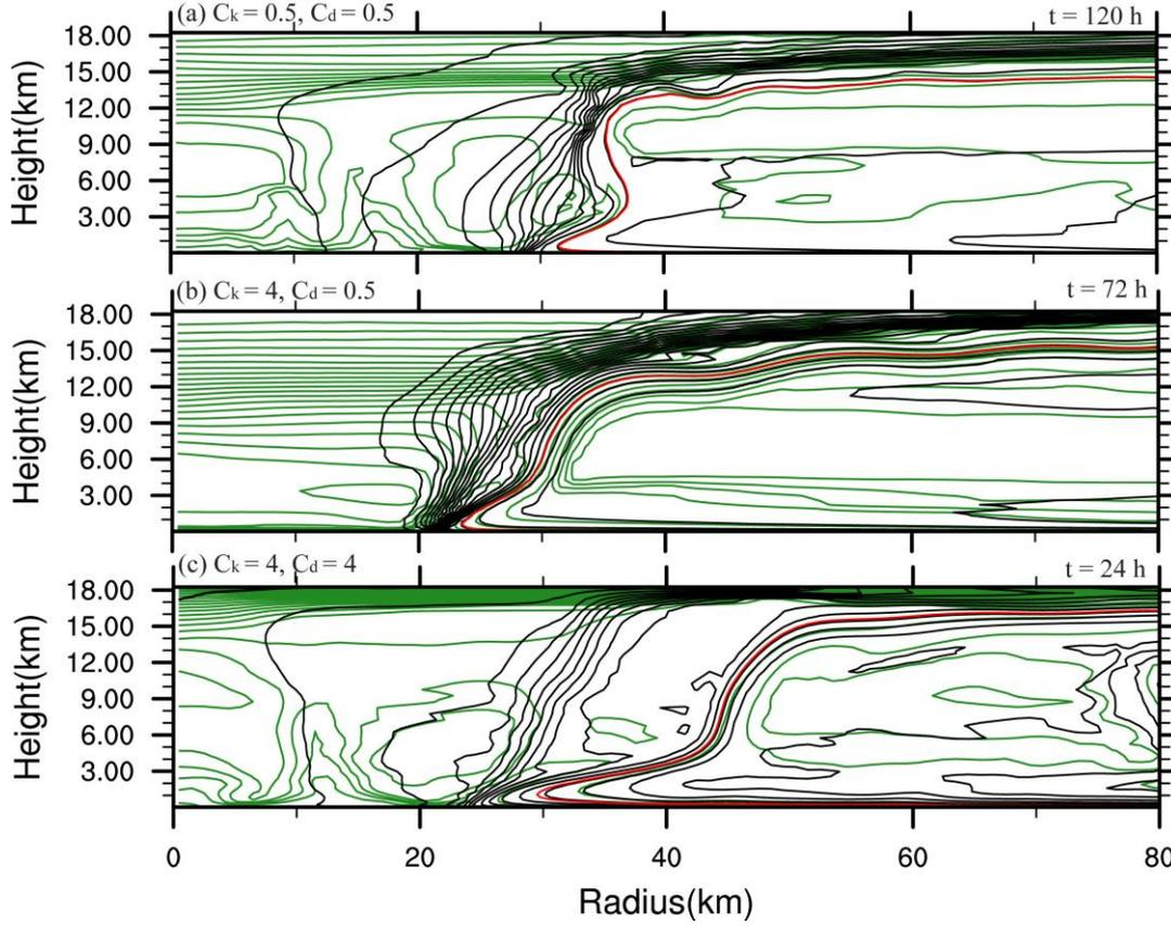
Fig. 2. Entropy  $s$  (contour interval =  $10 \text{ J kg}^{-1} \text{ K}^{-1}$ , green lines) and angular momentum  $M$  (contour interval =  $0.2 \times 10^6 \text{ m}^2 \text{ s}^{-1}$ , black lines) from the experiment with a)  $C_k = C_d = 0.5 \times 10^{-3}$ , b)  $C_k = 4 \times 10^{-3}$ ,  $C_d = 0.5 \times 10^{-3}$  and c)  $C_k = C_d = 4 \times 10^{-3}$ . The red line is the  $M$  surface that passes through the location of maximum tangential wind.
