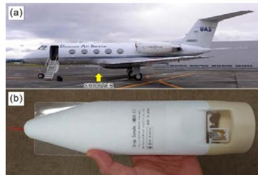
**Fig. 1** Photographs of (a) the Gulfstream-II jet and (b) a Meisei iMDS-17 dropsonde.
