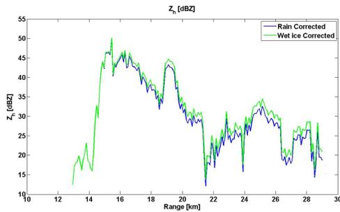
Figure 6:  $Z_h(X)$  for rain and wet ice attenuation corrected range profiles at  $58^\circ$  in azimuth.
