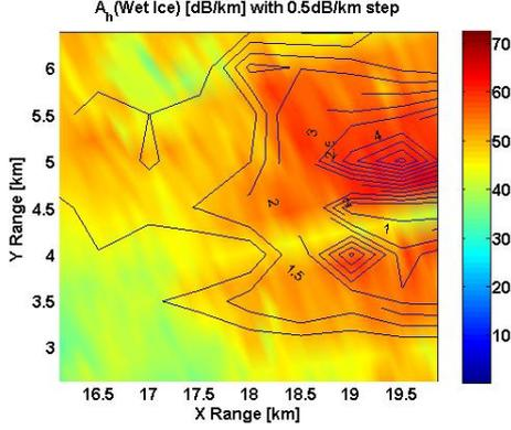
Figure 1: Contours of specific attenuation  $A_h^{wet-ice}(X)$  overlaid with wet ice corrected  $Z_h$  at X-band. PPI scan at  $12.25^\circ$  in elevation.
