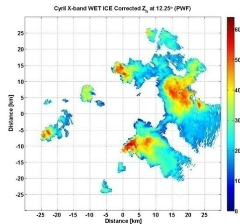
Figure 4: Wet ice attenuation corrected  $Z_h(X)$  PPI scan at  $12.25^\circ$
