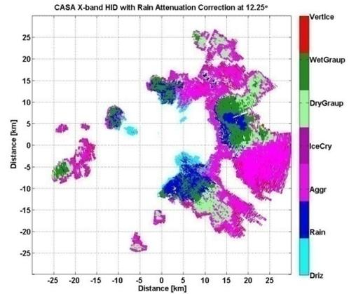
Figure 3: HID results for the event with all the classifications included. Rain induced attenuation corrected data at X-band was used here.
