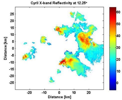
Figure 2: CASA Cyril CYR  $Z_h$  corrected for rain. PPI scan at  $12.25^\circ$  in elevation.
