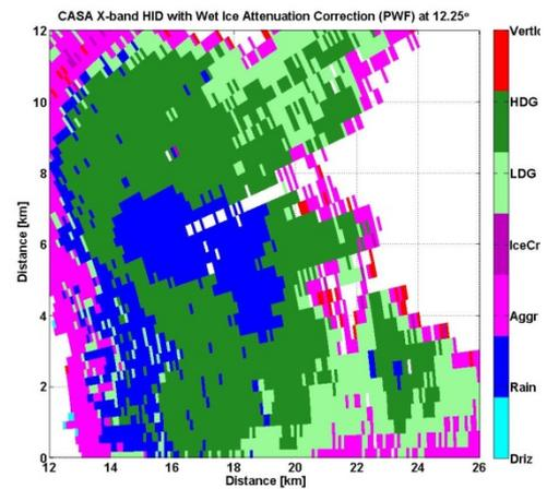
Figure 8: HID using the  $Z_h(X)$  corrected for wet ice using the PWF method.
