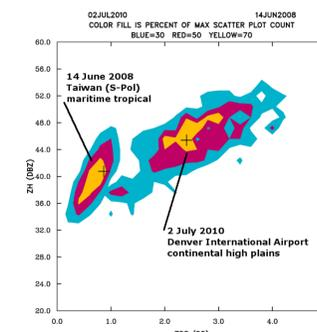
The two plots above show the same PPI data plotted in  $Z$  vs.  $Z_{dr}$  space; a polarimetric variable combination that has also been used for rain characterization (JPOLE, 2003). The separation between the two rain regimes is less distinct in the  $Z$  vs.  $Z_{dr}$  domain.
