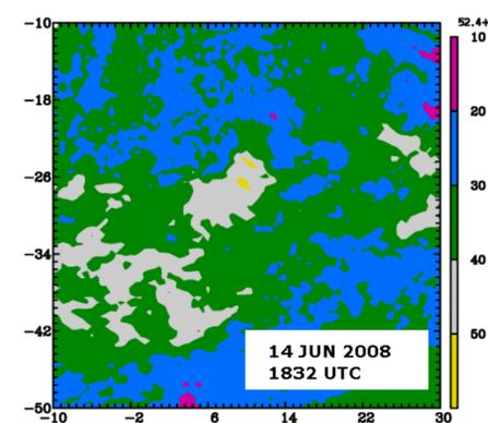
Above: Example gridded PPI plots of the reflectivity data (in dBZ) from the three cases. Axes units are in km from the radar.
