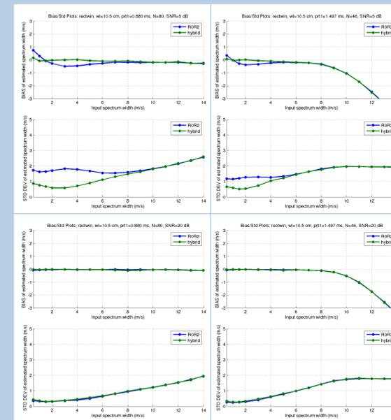
FIGURE 4: Bias and standard deviation of R0/R2 and HSW for 5 (top) and 20 (bottom) dB SNR, for 2 different operational modes (left/right).
