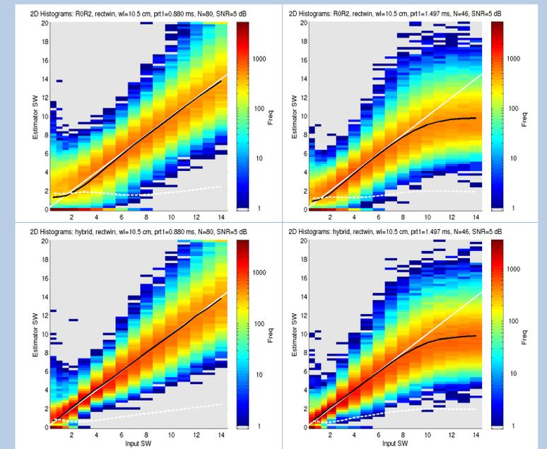
FIGURE 5: 2-D histograms of R0/R2 (top) and HSW (bottom) for 5 dB SNR, for 2 different operational modes (left/right).
