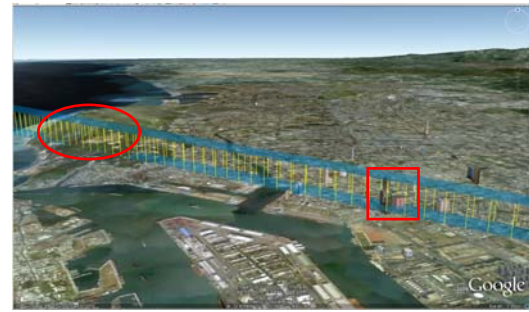
FIG.4. Radar beam propagation path of SPOL in Taiwan at the azimuth of 304.5^\circ and the elevation angle of 0.5^\circ . Two high rise buildings and mountains blocking the radar beam are marked by the red box and ellipse respectively. The two blue rays represent the radar beamwidth of 0.91^\circ . The yellow lines divide the path into radar gates with width of 150 m.
