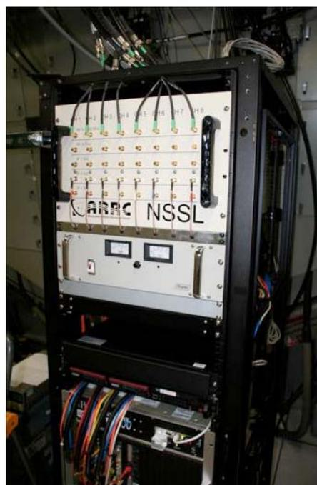
Figure 1. A picture of the new multi-channel receiver instrument rack installed at the National Weather Radar Testbed.
