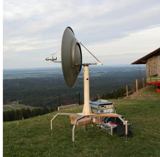
Figure 2: The transmitter dish/feed assembly.
