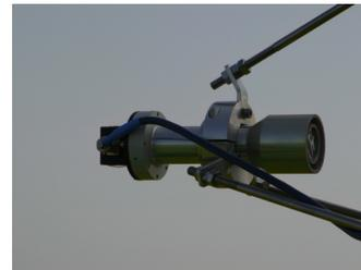
Figure 3: The single-pol feed of the transmitter dish.
