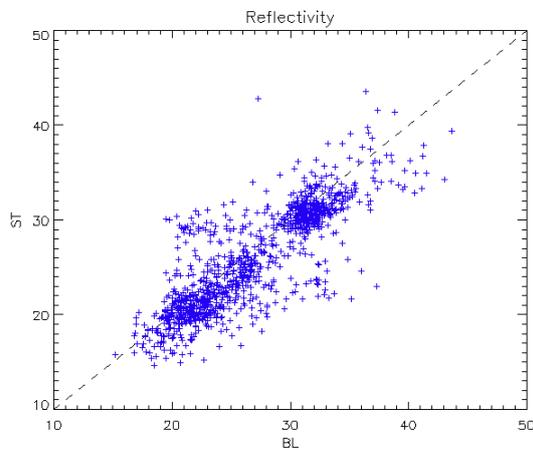
**Figure 8 Scatter plot showing the reflectivity measured on the BP BL, against that measured on the BP ST**
