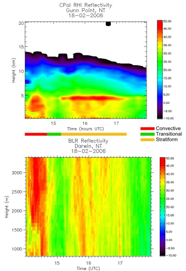
**Figure 1 CPOL RHI (top) and profiler cross-section (bottom) of reflectivity. The storm has been classified as indicated by the legend between the images, and consisted of a convective line, with trailing stratiform precipitation, separated by a transition region. (note the difference in height scales)**
