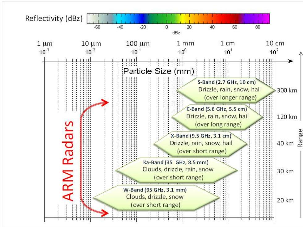
Figure 2: Diagram showing the the observational capability of ARM radars. ARM radar cover the whole range of hydrometeors ranging from small cloud droplets (W-band) to big rain drops and hail (C-band).
