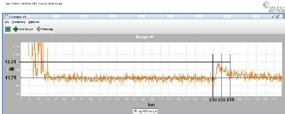
Fig. 2: Distance Measurement. Amplitude is normalized raw logarithmic power, without noise correction
