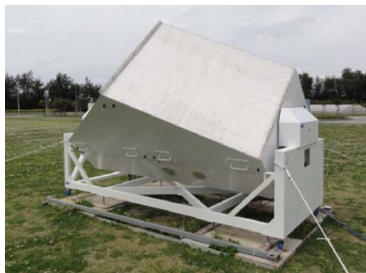
Fig. 2. Outlook of the Ka-radar with the beam 45 degree elevation
