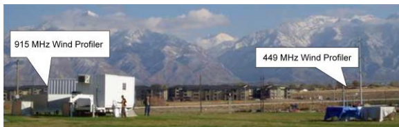
Figure 3: Close deployment of both a standard 915 MHz DBS wind profiler and the prototype 3-antenna 449 MHz wind profiler.
