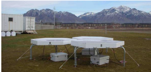
Figure 2: Prototype 3-antenna 449 MHz wind profiler, including radomes, in Salt Lake City, UT for PCAPS, November 2010.
