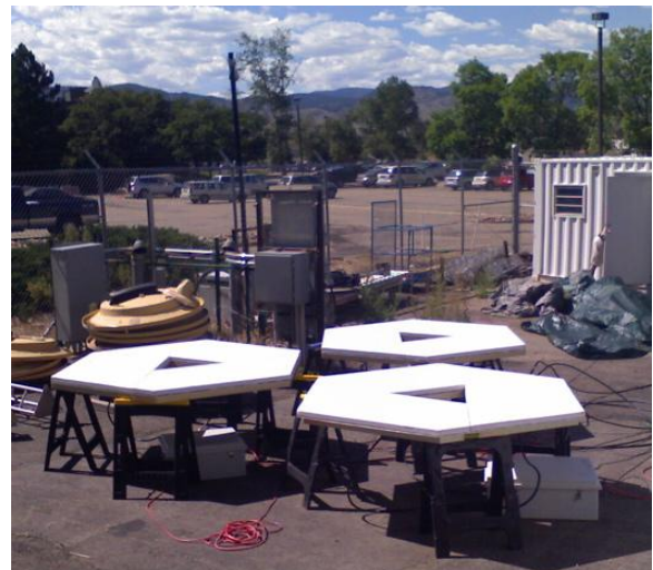
Figure 1: Prototype 3-antenna 449 MHz wind profiler in Boulder, CO, early 2010.
