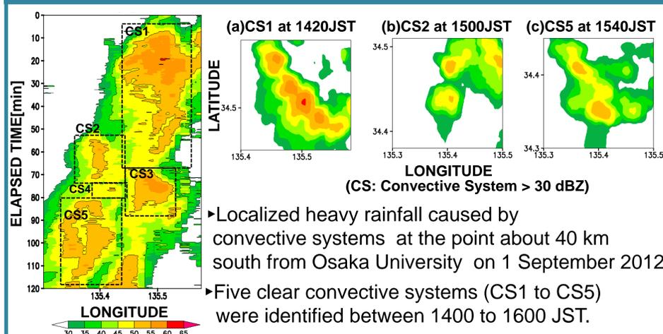
Localized heavy rainfall caused by convective systems at the point about 40 km south from Osaka University on 1 September 2012
