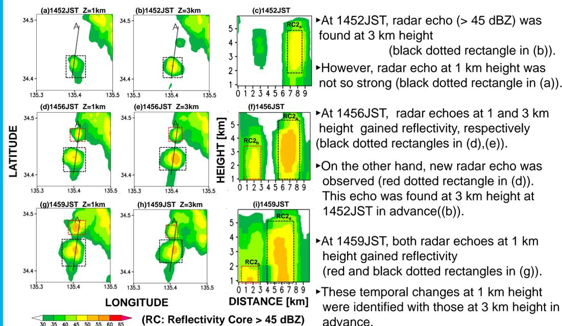
At 1452JST, radar echo (> 45 dBZ) was found at 3 km height (black dotted rectangle in (b)). However, radar echo at 1 km height was not so strong (black dotted rectangle in (a)).
