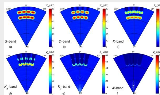
**Figure 2:** The frequency effect. (a,b) Antenna diameter  $D_a = 2$  m, and (c,d,e,f)  $D_a = 0.8$  m. All convective towers contain hail (here  $R_h = 40$  mm  $h^{-1}$ )
