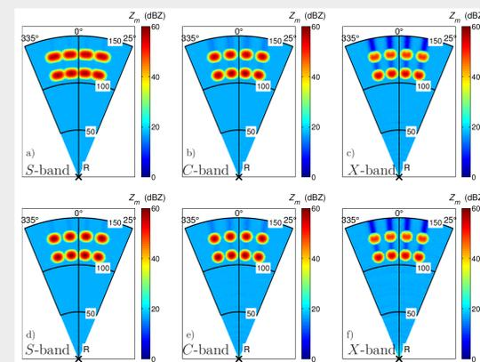
**Figure 3:** The  $\theta_{3dB}$  effect. PPI view simulation of the measured reflectivity  $Z_m$  in a mesoscale system at various frequency bands:  $S$  (a,d),  $C$  (b,e),  $X$  (c,f), with a radar antenna size of 2 m (a,b,c) and of 4 m (d,e,f).
