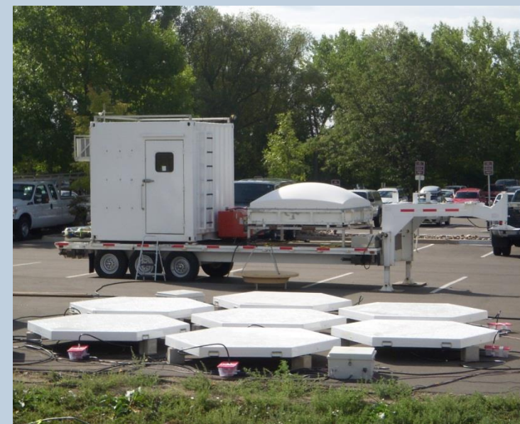
NCAR profilers Foreground: new 7-gated modular 449 MHz profiler Background: mobile 915 MHz profiler
