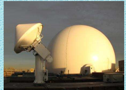
Picture of TropiNet radar at CSU CHILL under testing and calibration campaign
