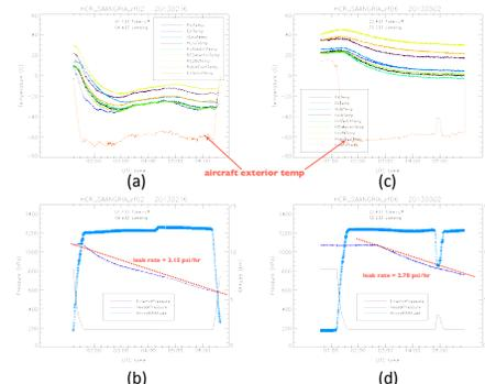
Figure 3. (a,b) HCR temperature and pressure profiles during flight #2. (c,d) increased system temperature and reduced leak rate.
