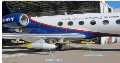
Figure 1. HCR installed on NCAR GV aircraft. Front large pod: HIAPER Cloud Radar; rear large pod: counter weight.
