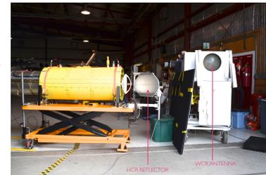
Figure 6. WCR/HCR intercomparison setup.
