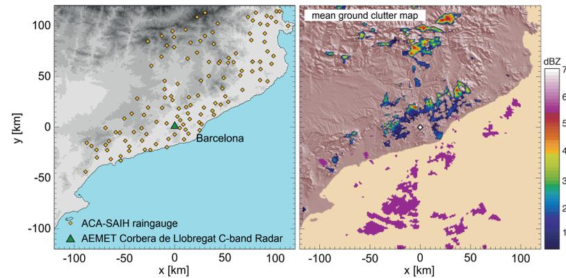
125 rain gauges of the Catalan Water Agency have been used in the validation of the methodology.
