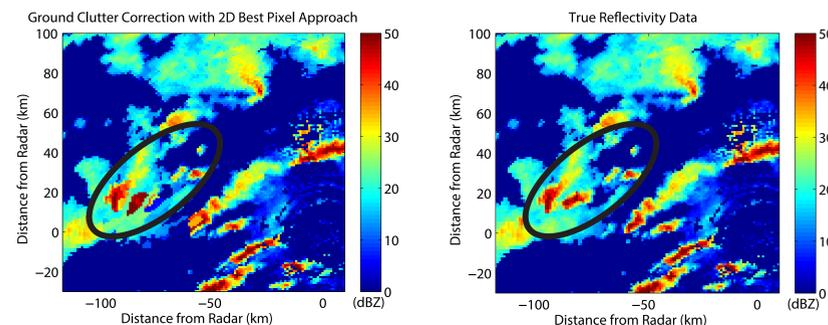
Replace each pixel within a region of false (created) ground clutter with an uncluttered pixel from the same radar scan that has the lowest available variance (left) and compare with the true reflectivity data (right) to evaluate the “best pixel” method.
