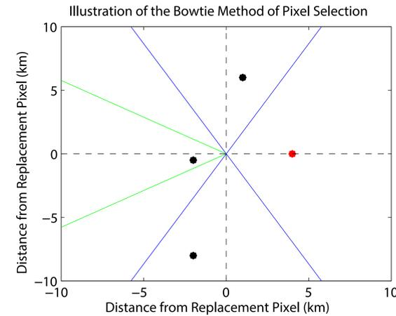
We developed a “smart” ordinary kriging method that reduces the number of spatially redundant pixels being averaged by requiring that each pixel be at least 30 degrees from any other pixel.
