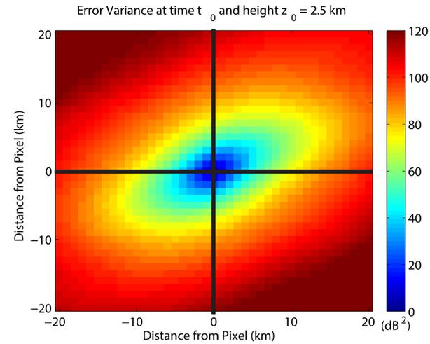
A variogram (depiction of the mean variance as a function of distance from a pixel contaminated by ground clutter) for a convective precipitation event at the McGill radar. This figure gives a 2D picture of the error that would result if we were to replace a contaminated pixel with another pixel from its surroundings.
