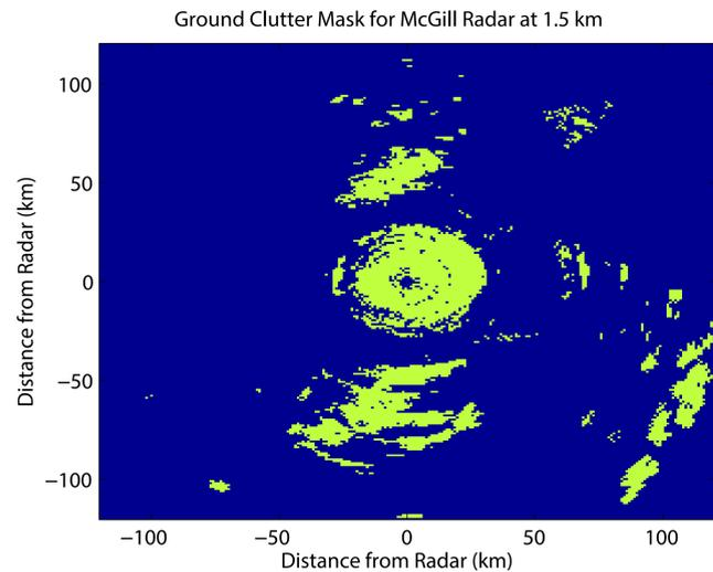
Actual ground clutter present at the McGill radar (green pixels indicate ground clutter, blue pixels indicate uncluttered data). Each pixel is 1 km x 1 km.
