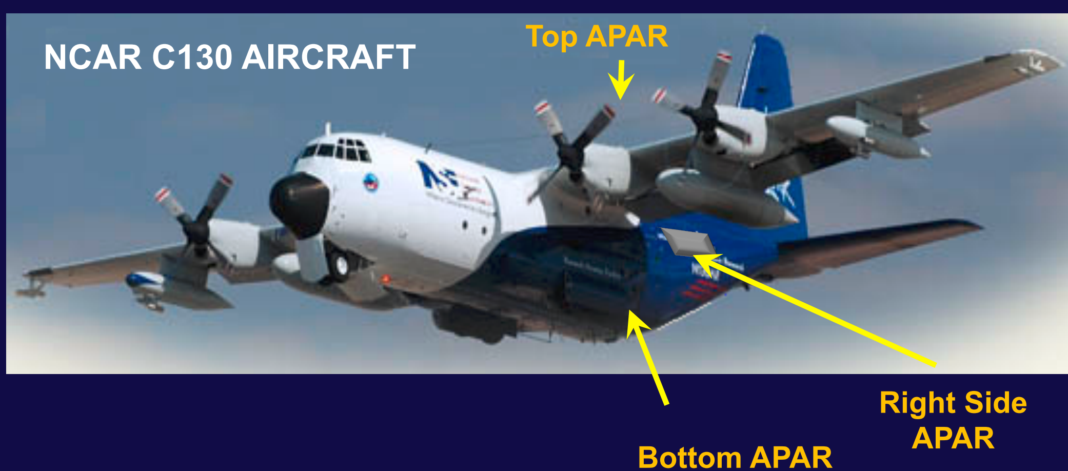
Figure 1. Proposed configuration of C-band active electronically scanned array (AESA) radars on C-130. Four AESA radars are strategically mounted on the fuselage of the NSF/NCAR C-130 turboprop aircraft
